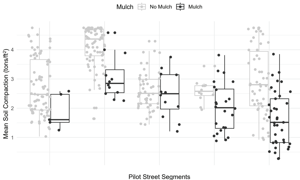
Figure S5. Pilot soil compaction data and presence of mulch for a subset of Chicago segments in 2022 ( n = 367 trees). Each pair of box-plots (grey and black) refers to a different pilot street segment in Chicago. Soil compaction was measured with a pocket penetrometer at 6 points around the base of the trunk, within the canopy drip line. The presence or absence of mulch was noted as part of field data collection.
