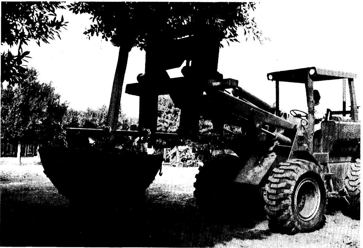
Figure 3. Tree-Porter dug root ball of 80" on 7" caliper Ficus is lifted by a nursery fork-lift unit that also loads trucks. Tree-Porter (background) takes hydraulic power from a small nursery tractor. Hydraulic jack-hammer keeps digging in hard and stony ground.
