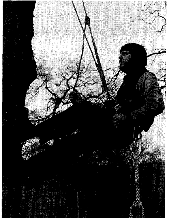
Fig. 6. The prussik knot in action taking the climber's weight, the remainder of the rope being slack and the other end of the loop system parked on the side for ease of illustration. It would normally be parked on the front of the harness.
