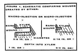
sertion tool with an 11/64" diameter bit in a portable drill to make the wound in the root flare. The resulting drill wound is cleaner edged and the depth is under more precise control. These factors greatly facilitate wound closure because the degree of injury resulting from the mechanical wound is minimized. In addition the injected material is more rapidly translocated away from the injection site (4).
