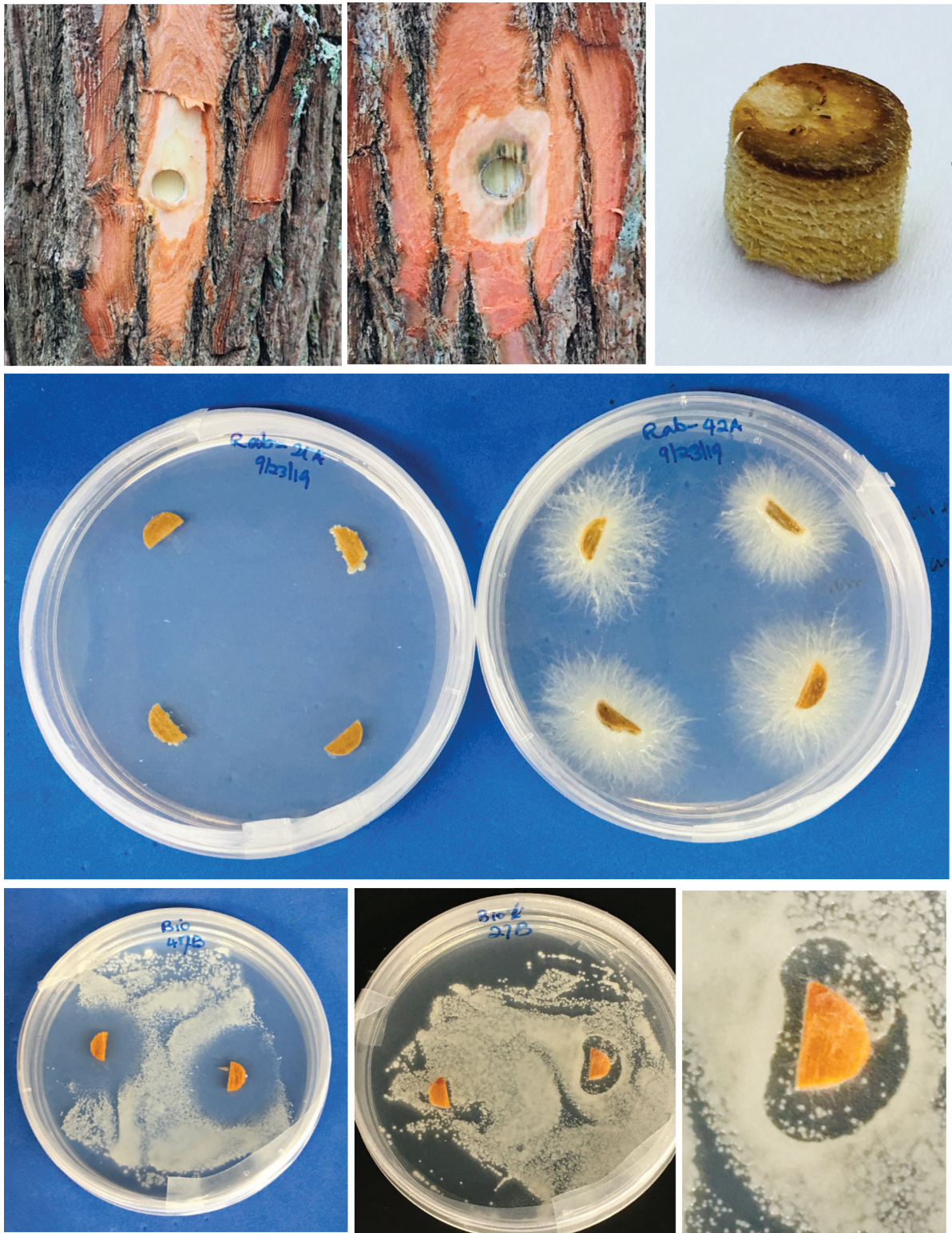
Figure 1. Tissue-sample discs collected from inoculated and noninoculated sassafras trees (top); tissue discs plated on potato dextrose agar (PDA) for re-isolation of H. lauricola (middle); and inhibition zones from the evaluation of the movement and retention of propiconazole in sassafras tissue samples on PDA pre-inoculated with spores of H. lauricola (bottom).
