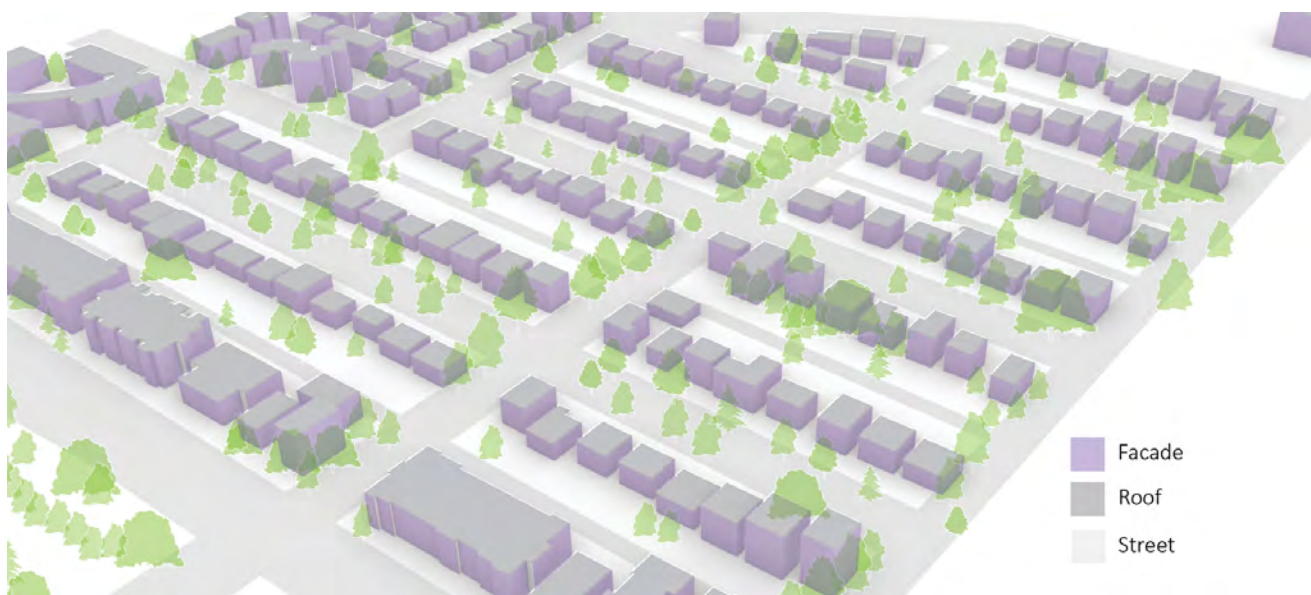
Figure 3. Surfaces (façades, roofs, and streets) simulated in this work. The amount of solar radiation with and without urban canopies will be generated and compared for each surface type.
