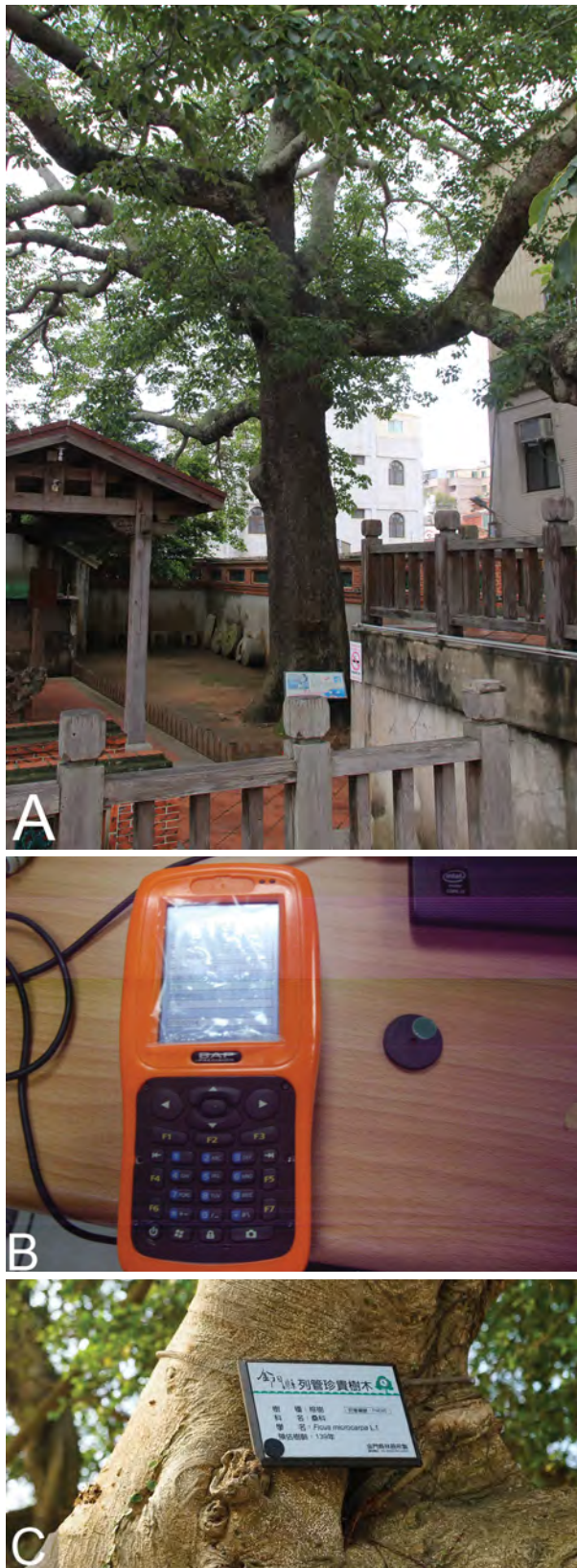
Figure 5. (A) Protected tree; (B) RFID reader and tag; (C) Tree tag with detailed information.
