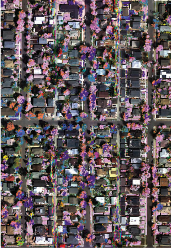
Figure 3. RPA image resolution and plant health. Proprietary early machine learning–derived plant health algorithm at neighborhood scale overlaid with visual imagery. Flight level: 120 m above ground level. The resolution of tree crowns less than 1-m diameter is detectable. Location: Denver, Colorado, USA.
