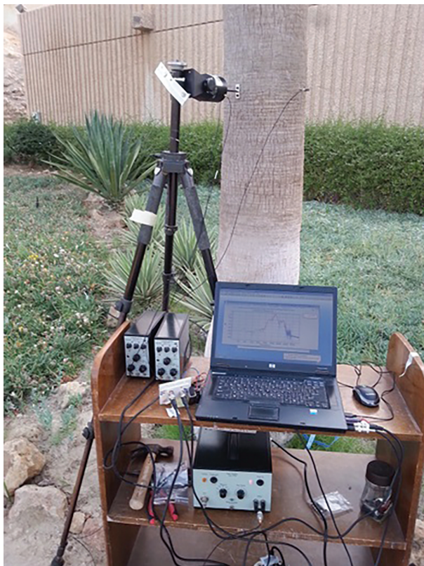
Figure 2. Photograph of the experimental measurement set-up used for sensing the ovalling mode on a palm tree trunk.
