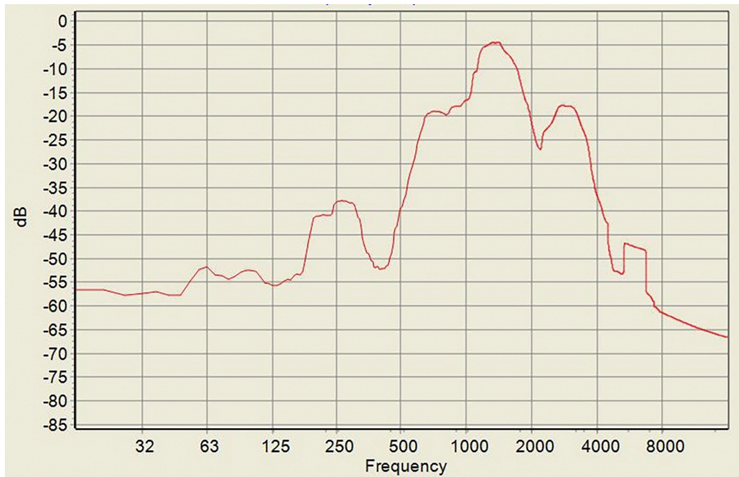
Figure 9. Amplitude of the transfer function, i.e., the transform of the impulse response in the frequency domain, smoothed curve.
