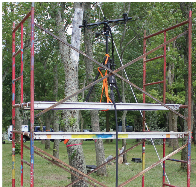
Figure 1. Digital image correlation samples with stereo camera system mounted on a scaffolding. The branch in the background has been painted white with black speckles for strain mapping.
