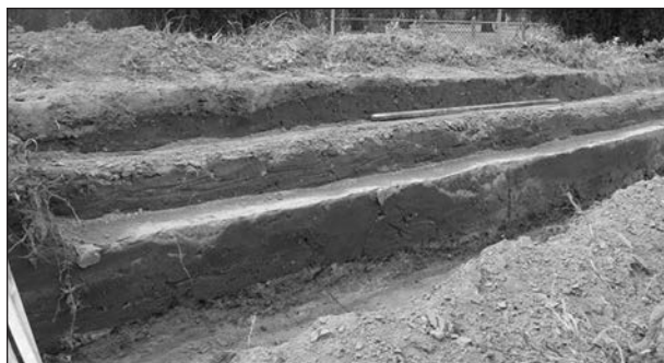
Figure 3. Prepared stepped trenches for Experiments 1 and 2 at 200 mm, 400 mm, and 800 mm depth.
