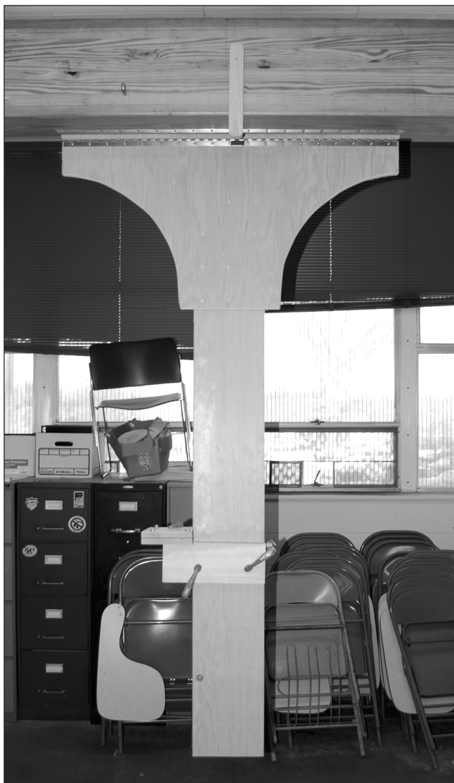
Figure 2. Pendulum attached to beam; the jig that held blades (see Figure 3) is attached to the pendulum with clamps visible just below the midpoint of the pendulum.
