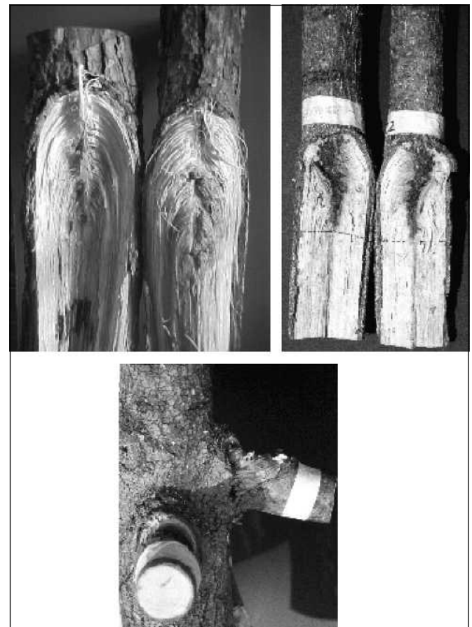
Figure 4. Examples of the three failure modes clockwise from top left: embedded branch failure on a white oak (not part of this study), flat surface failure on a sawtooth oak with included bark, ball in socket failure on a callery pear.
