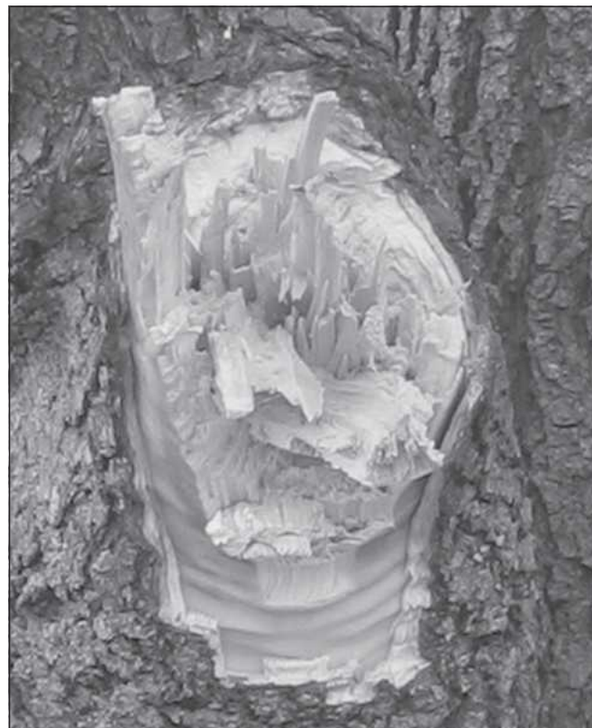
Figure 5. Failure that was difficult to categorize as branch or attachment based on the definitions presented in the text. The initial failure appears to occur at the apex of the attachment but below that most of the failed fibers are from the branch not the trunk.
