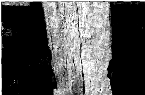
Figure 6. No changes of the wood are visible in the area where belt and tree were in contact.
