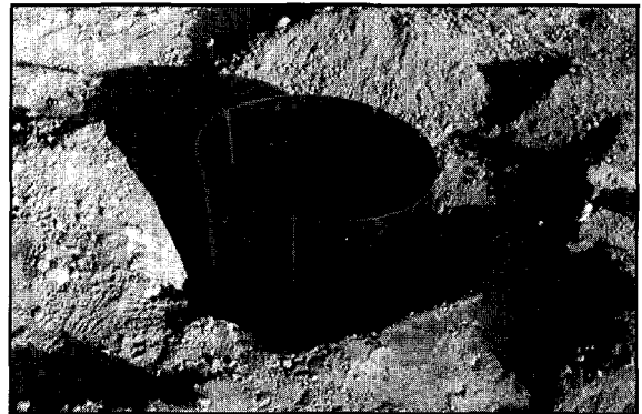
Figure 1. Circling barriers are used to protect hardscape elements from damage by deflecting tree roots vertically to the bottom of the barrier. In this study, four commercially available root barriers were used to examine root development inside and outside barriers.
