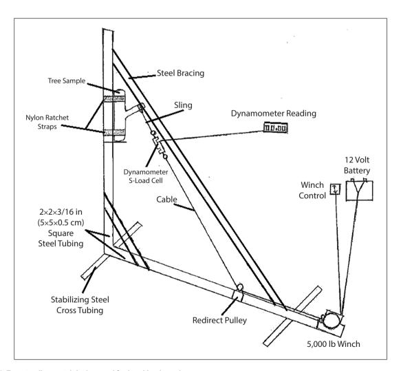
Figure 1. Freestanding metal device used for breaking branches.
