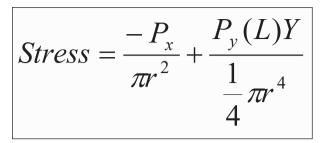
Figure 2. Equation for calculating stress on the lower side of the branch.
