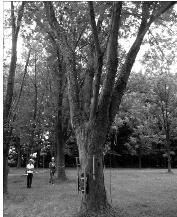
Figure 1. Silver maple ( Acer saccharinum ) with four codominant branches and strain meter attached to the trunk. Location: Davey Tree reserve, Shalersville, Ohio, U.S. (Note: the fifth smallest branch shown was removed prior to testing).
