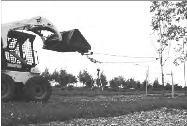
Figure 3. Configuration of pulling equipment and dynamometer used to evaluate tree stabilization systems (staking shown) on field-grown, balled and burlapped white ash ( Fraxinus americana L. 'Autumn Purple').
