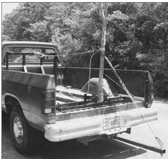
Figure 2. Truck-mounted tree sled used for measuring wind-induced bending moment of white ash ( Fraxinus americana L. 'Autumn Purple') from 0 to 24.5 m/s (0 to 55 mph).
