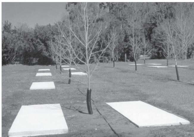
Figure 1. One tree was planted between sidewalk sections with various vertical root barriers on the tree side of the walk, or gravel under the walk, or a control without a barrier.
