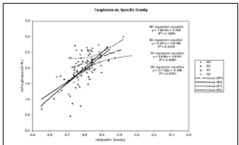
**Figure 4. Scatter diagram and best fit lines from regression of each sample's toughness (natural log transformed) on sample specific gravity (natural log transformed). The dashed line corresponds to W1 samples—the only samples where specific gravity did not significantly account for toughness variation. The dotted lines indicate upper and lower 95% confidence limits for the W1 regression line.**
