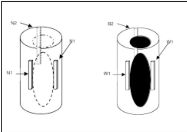
**Figure 3.** Line drawings show locations of samples taken from normal wood (left) and woundwood bolts from each tree. The dashed lines serve to reference the woundwood samples from the woundwood bolt.
