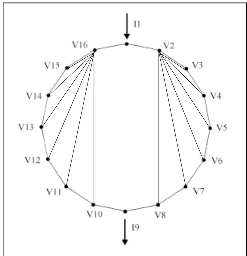
**Figure 2. Data acquisition scheme of electric tomography. I: source electrodes; V: receiver electrodes. This picture shows current immission between electrode 1 and 9 and measurement of the potential difference among all other electrodes.**
