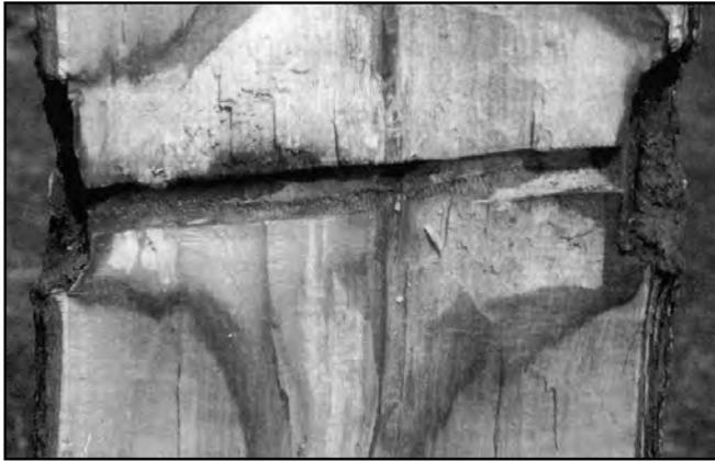
**Figure 3. Longitudinal view of discoloration and decay extending from drill hole for hardware installation (note countersinking of washers into wood) (Stobbe et al. 2000).**
