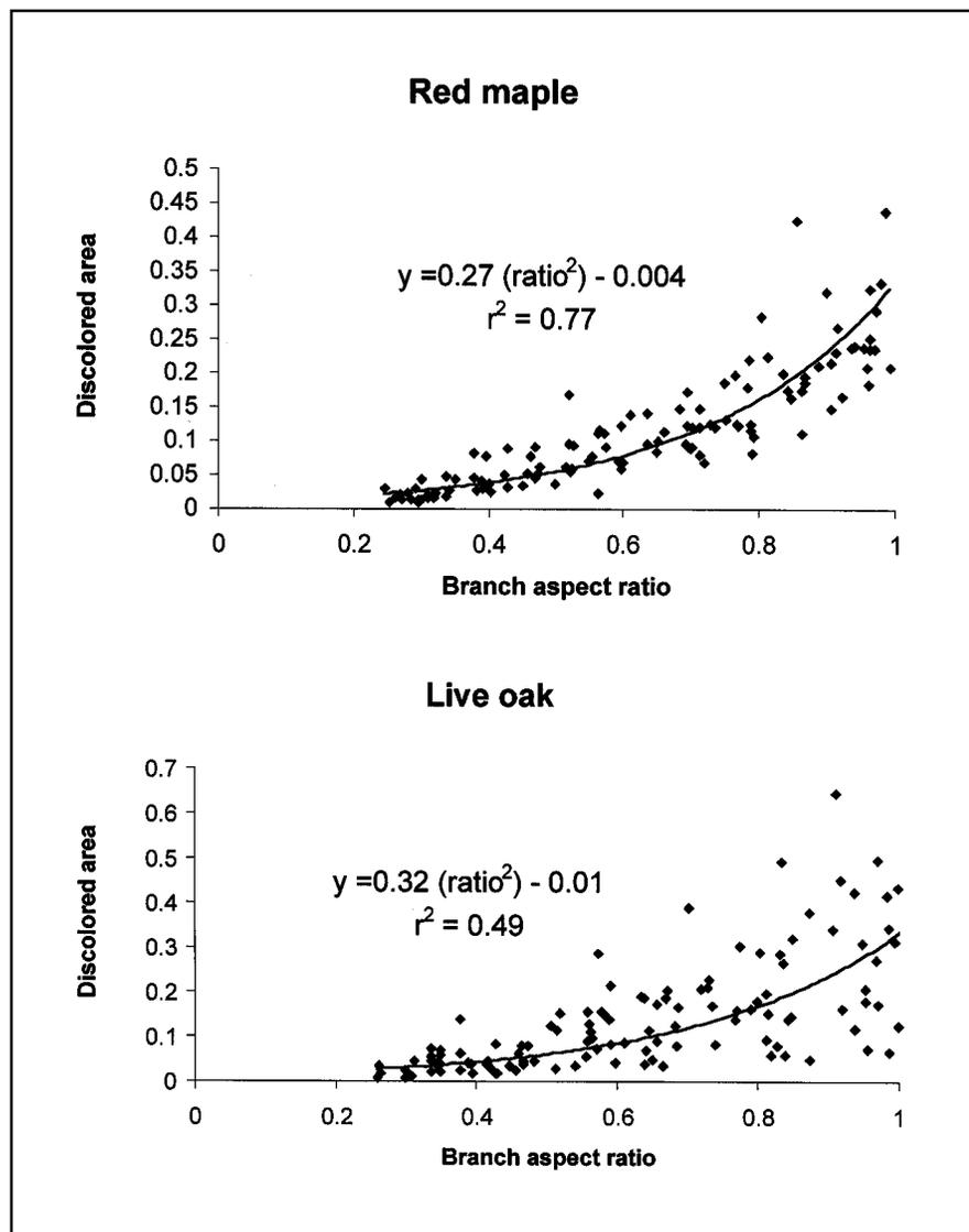
**Figure 2.** The impact of aspect ratio on trunk discoloration [ $\log_{10}$  discolored area ( $\text{cm}^2$ )  $\div$  trunk cross-section area ( $\text{cm}^2$ )] that developed in the medial longitudinal plane of dissected branch junctions four months after branch removal.
