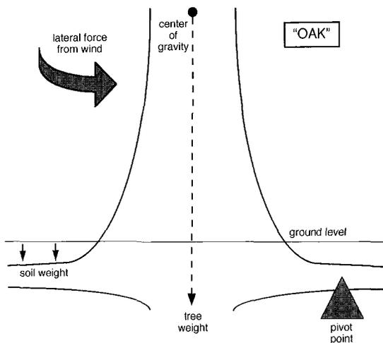
Figure 1. The factors involved in compressive buttressing.
