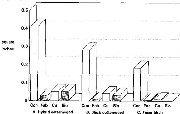
**Figure 6.** Cross-sectional area of three largest roots in soil volumes 0.5 foot beyond the 1- by 2-foot treatment zones for A) hybrid cottonwood, B) black cottonwood, and C) paper birch. Treatments were control (Con), nylon fabric (Fab), copper screen (Cu), and Biobarrier (Bio).
