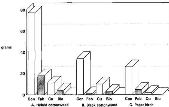
**Figure 5.** Dry weights of roots in soil volumes 0.5 foot beyond the 1- by 2-foot treatment zones for A) hybrid cottonwood, B) black cottonwood, and C) paper birch. Treatments were control (Con), nylon fabric (Fab), copper screen (Cu), and Biobarrier (Bio).
