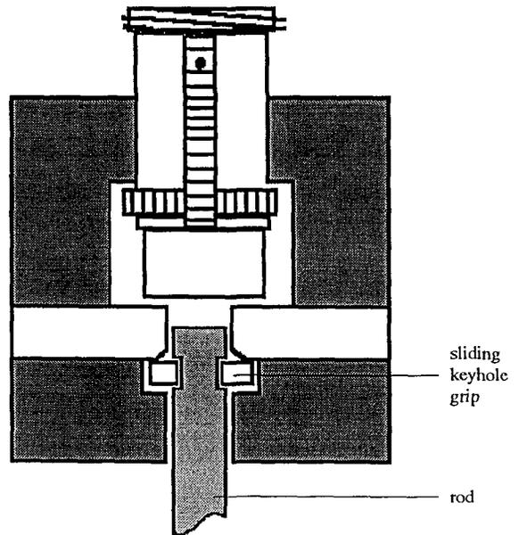
**Figure 4: Detail of rod coupling on extraction jack.**
