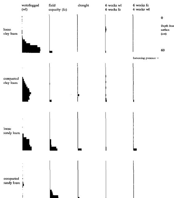
**Figure 2: Presence of smooth black corrosion on steel rods after three months under five soil moisture regimes.**
