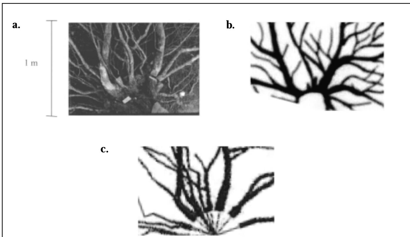
Figure 6. Comparison of one 1 m<sup>2</sup> (10.8 ft<sup>2</sup>) transect from the root system of *Pinus nigra*, using images from (a) photograph, (b) GPR data, and (c) 2D reconstruction derived from digitized architecture data. The large lateral roots appear to be detected by GPR, as can be seen from both the photograph and the 2D digitized image.
