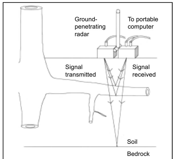
**Figure 1.** Schematic representation of a portable ground-penetrating radar (GPR) device. Tree roots are detected by an electromagnetic signal, as anomalies in the soil, and this information is transmitted in the form of travel time pulses to a portable computer.
