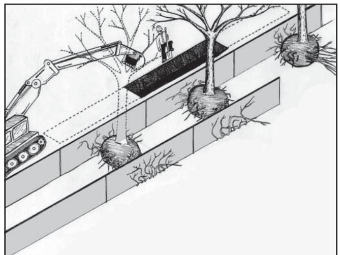
**Figure 1. Graphic representation of root excavation process.**
