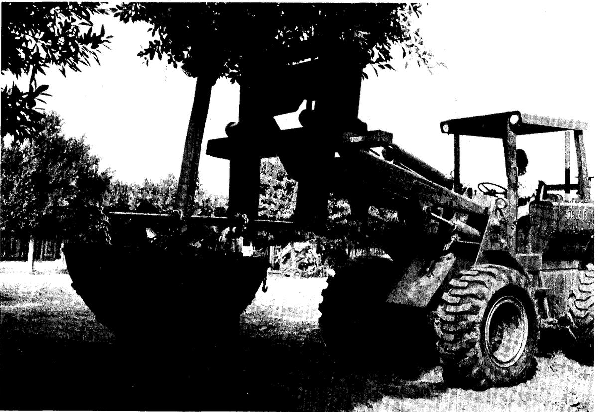
**Figure 3. Tree-Porter dug root ball of 80" on 7" caliper *Ficus* is lifted by a nursery fork-lift unit that also loads trucks. Tree-Porter (background) takes hydraulic power from a small nursery tractor. Hydraulic jack-hammer keeps digging in hard and stony ground.**
