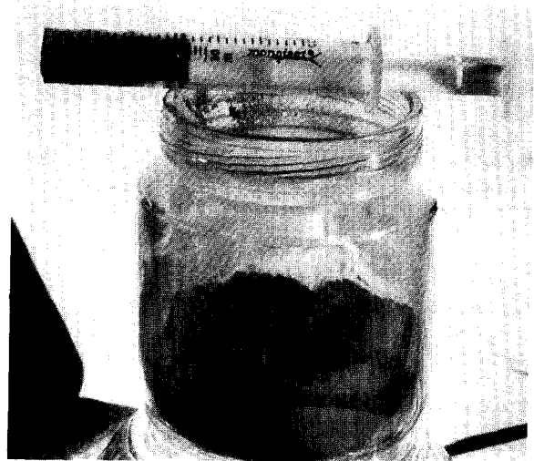
Fig. 2. A 3 ml plastic syringe with the tip end removed to facilitate loading with powdered ferric citrate.
