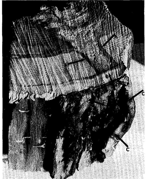
hole had been drilled into a central column of decay. When holes are drilled into decay, new decay will spread rapidly out around the edges of the new hole. New growth rings will compartmentalize the washer and give the rod holding power.
